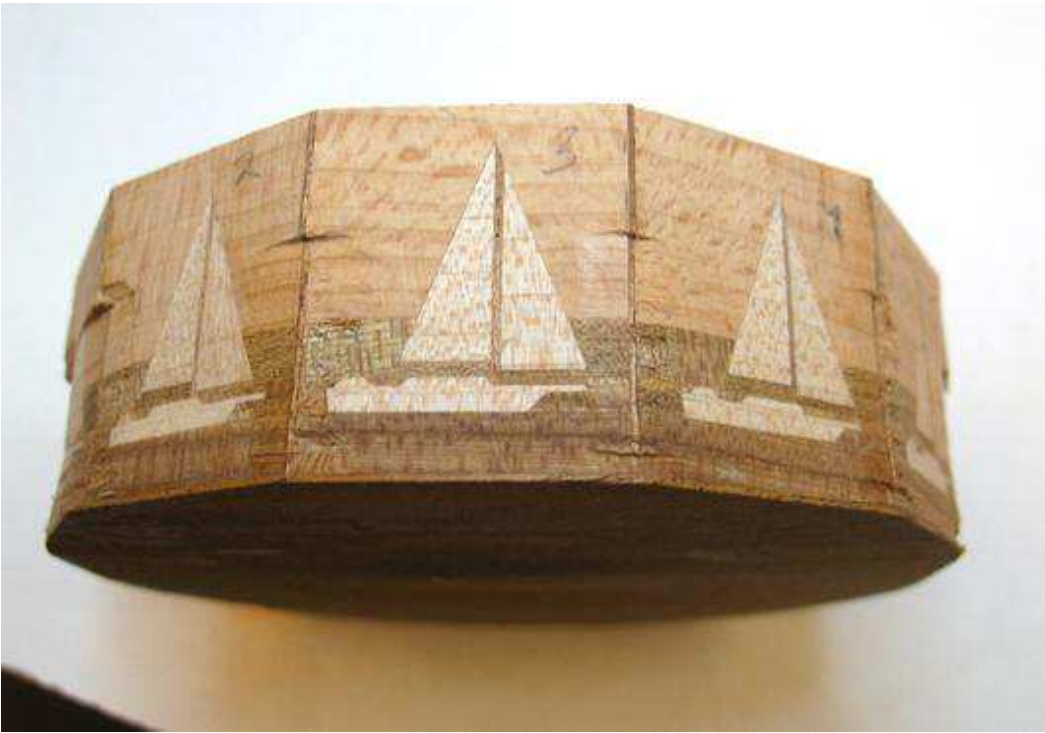
Miter angles are cut and sanded. The segments are then glued into a ring.
