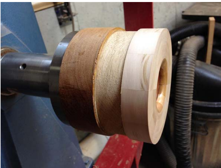
Photo 14 – After the bowl is completed and parted off the faceplate waste block, the floating disk recess can be used for exact centering of the bowl for reverse turning the base.
