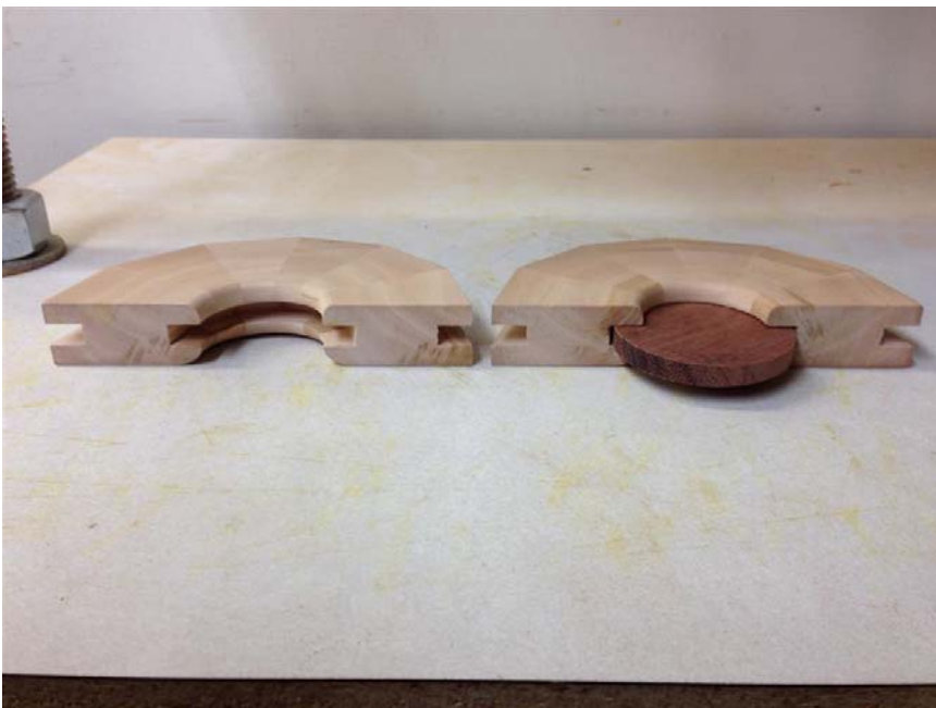
Photo 8 – The disk was made and fitted. The disk is about 1/16" loose on the OD and about .010" loose on the top/bottom in the slot. Top ring side is facing down.
