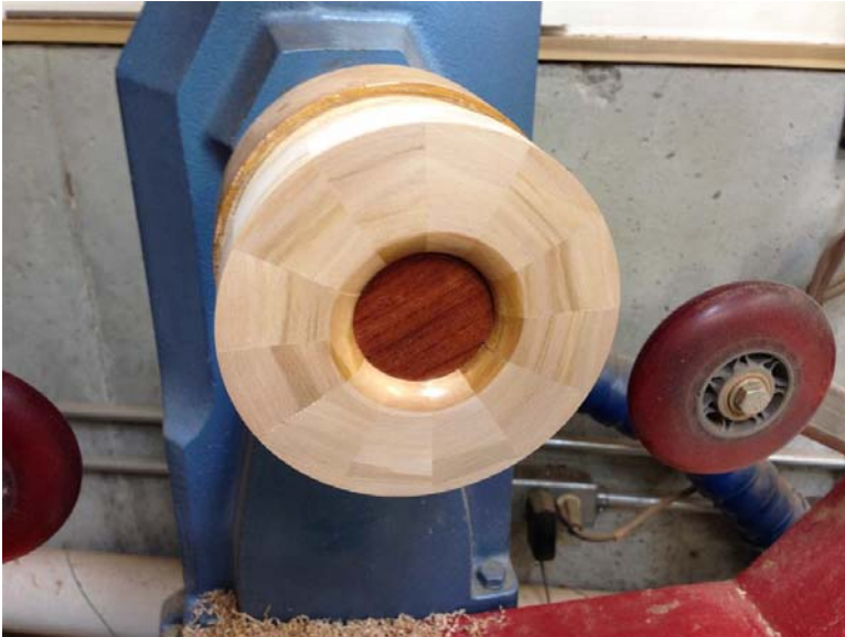
Photo 13 – The top side of the segment ring was faced off and flattened and the OD was rounded, removing the outer slot. The final ring dimensions are 4" OD by 1-1/2" ID.
