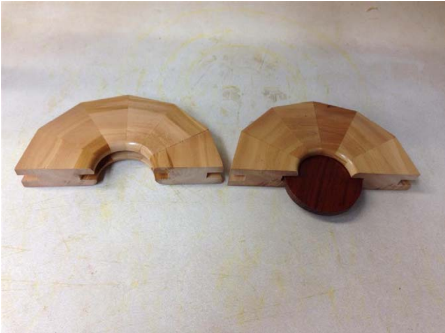
Photo 10 – All parts were separated and finished using lacquer. The disk was test fit again for looseness.
