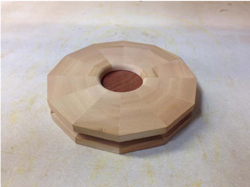
Photo 9 – The fit and disk looseness was tested with the ring halves rubber-banded together.
