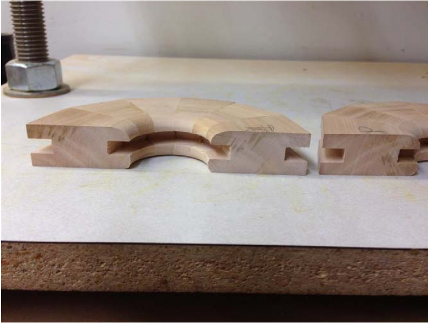
Photo 7 – The two rings halves have been separated to show the different curves of the inner side of the ring. Top ring side is facing up.
