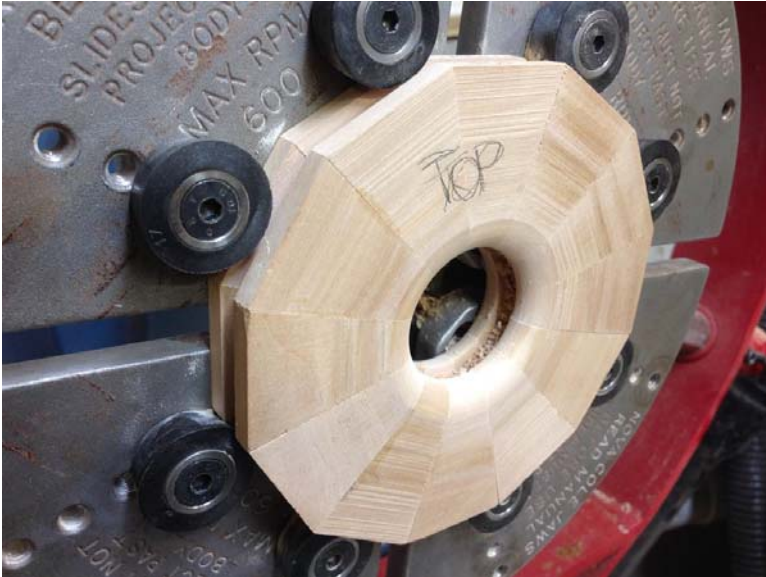
Photo 5 – The half rings were rubber banded together using the outer slots and clamped into a Cole jaw chuck. The top inner side of the ring has been turned round.
