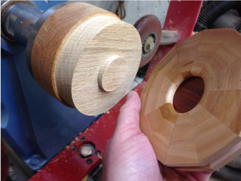
Photo 11 – The two ring halves were glued together, making sure the disk remained loose in the slot. A tenon was cut in the faceplate waste block to the exact ID of the floating disk recess. The tenon height has about 1/32" clearance to the floating disk (does not touch) to hold the faceplate end of the bowl in place as it is parted off the faceplate.
