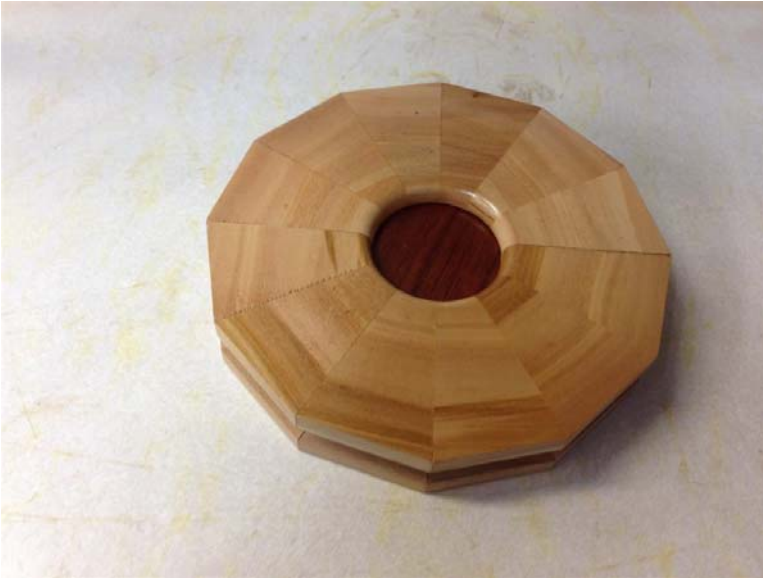
Photo 1 – Segmented base ring with floating disc. The slot for the floating disc was made using a table saw. Base ring and floating disc were finished with lacquer prior to assembly. The desired final segmented ring was 4" OD and 1-1/2" ID. Calculated dimensions including oversize board due to outside slot: Segment Edge Length 1.072", Board Width 1-3/4", Board Length 13".
