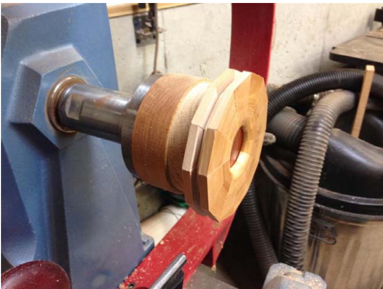
Photo 12 – The lacquer on the bottom side of the ring was sanded off and the ring was glued to the faceplate waste block.
