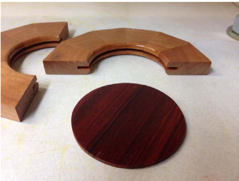
Photo 12 – All parts were separated and finished using lacquer. The disk was test fit again for looseness.
