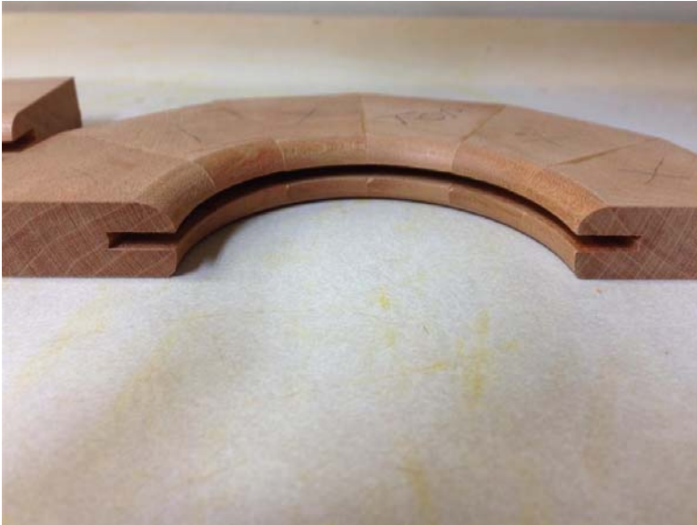
Photo 11 – The two rings halves have been separated to show the different curves of the inner side of the ring. Top ring side is facing up.
