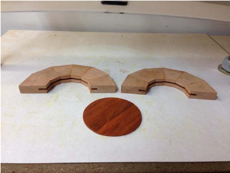
Photo 8 – The segments were glued together into two half rings. The segment top, marked with an X, is facing upwards. I sanded the half-ring butts to make the ring halves fit together perfectly. The disk was cut to about 1/16” radial clearance and sanded to a nice sliding fit, which is about .010” clearance.
