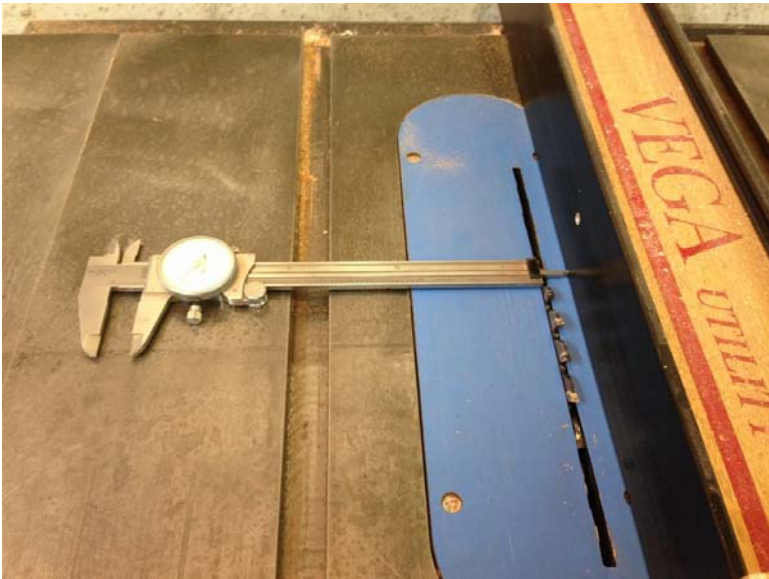
Photo 7 - The blade to fence dimension was set with a dial caliper.
