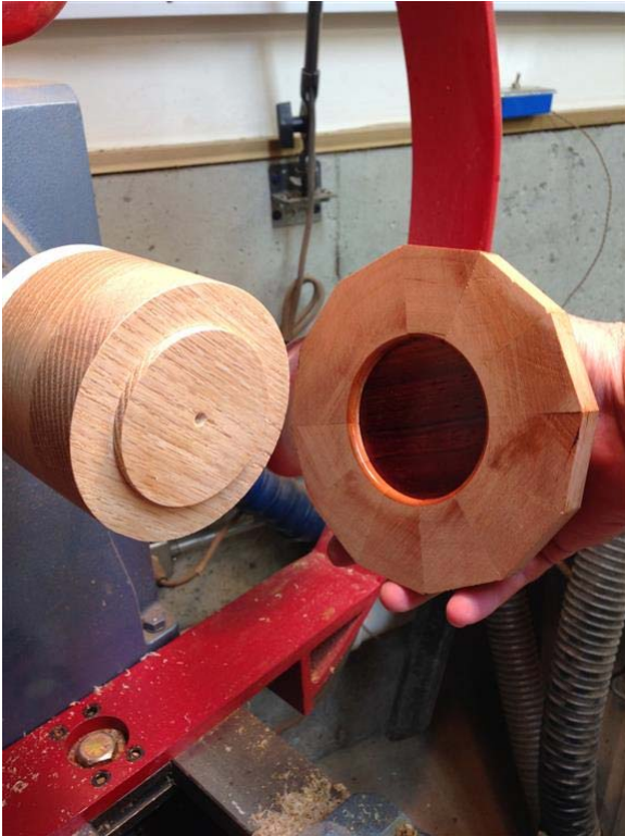
Photo 13 – The two ring halves were glued together, making sure the disk remained loose in the slot. A tenon was cut in the faceplate waste block to the exact ID of the floating disk recess. The tenon height has about 1/32'' clearance to the floating disk (does not touch) to hold the faceplate end of the bowl in place as it is parted off the faceplate.
