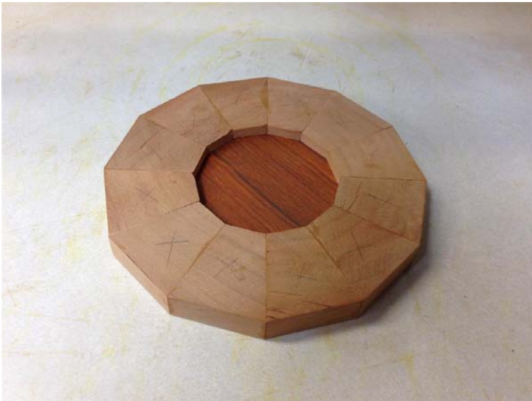
Photo 9 – Test fitting the segment ring and disk.
