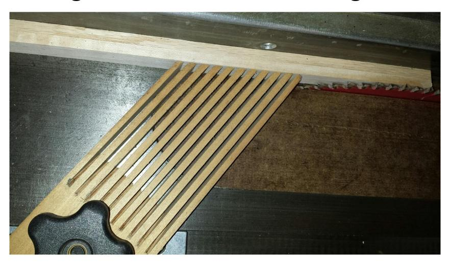
Sand or plane the strips to 3/8"x ¾"x 24." They will need to be the same size for later construction. ("V" grove)
