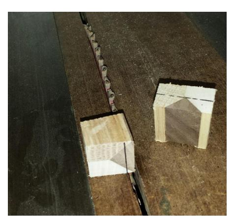
Trim off lower waste on 24" strip to 1/16" or less, all strips must be alike for ring glue-up later.
