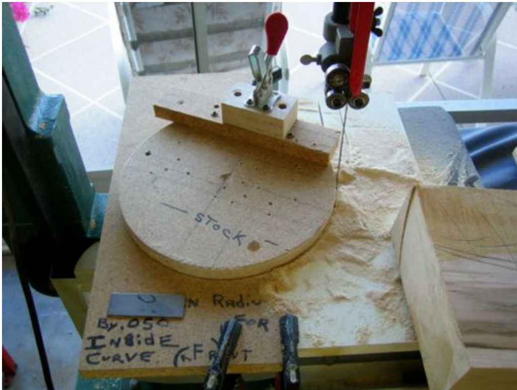
Bandsaw Fixture For cutting Curves. From the book Beyond the Basic Turning By Jack Cox
