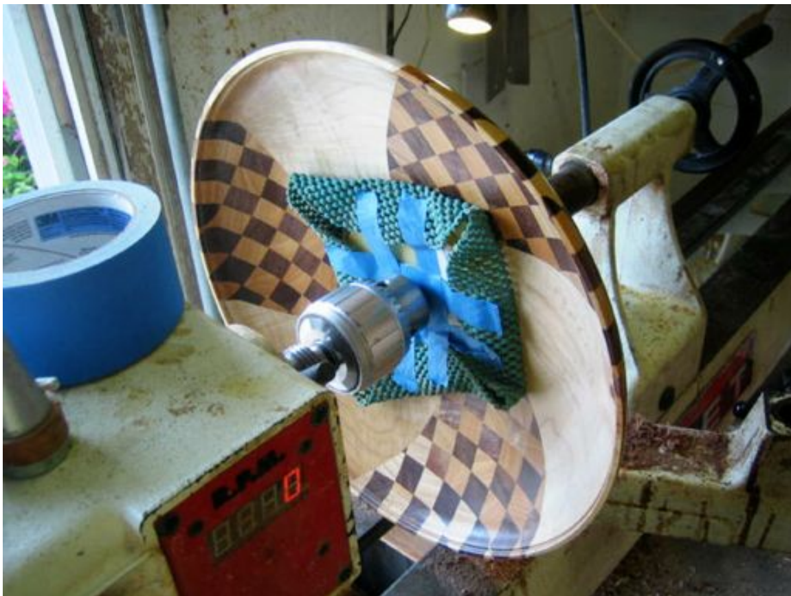
Set up for finishing the Bottom
