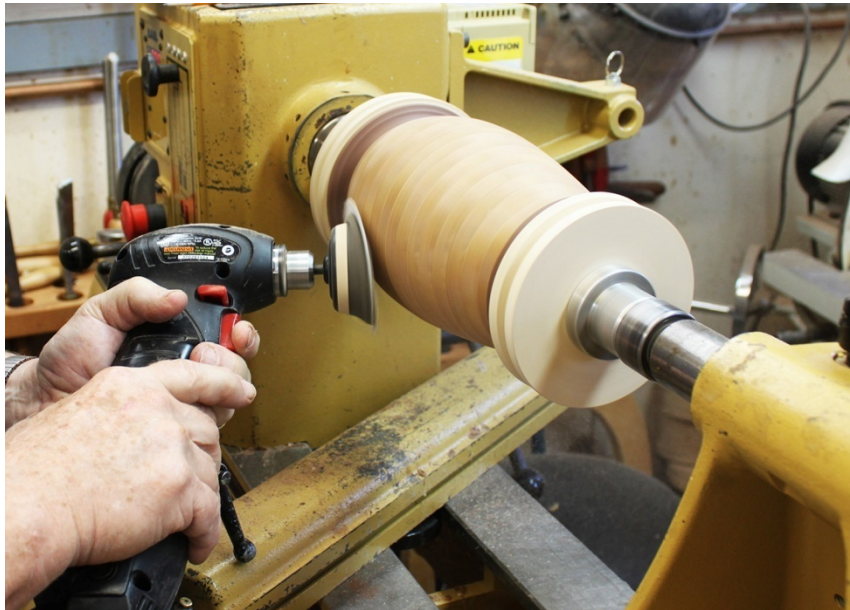
Sand joint area
