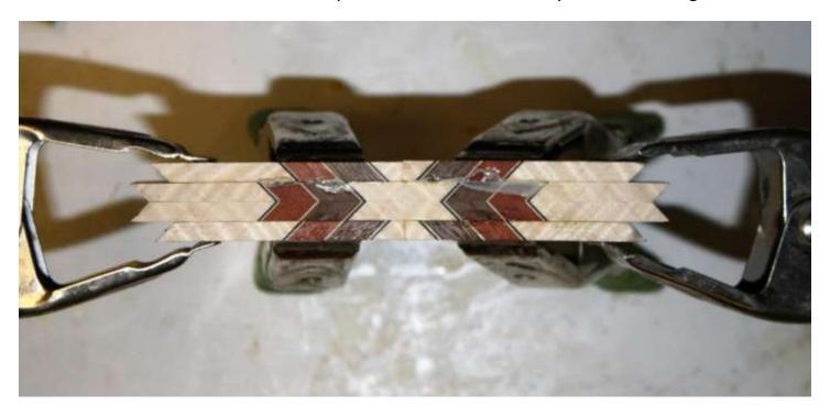
After these have dried we can sand both sides to ready the assembly for the next two layers.
