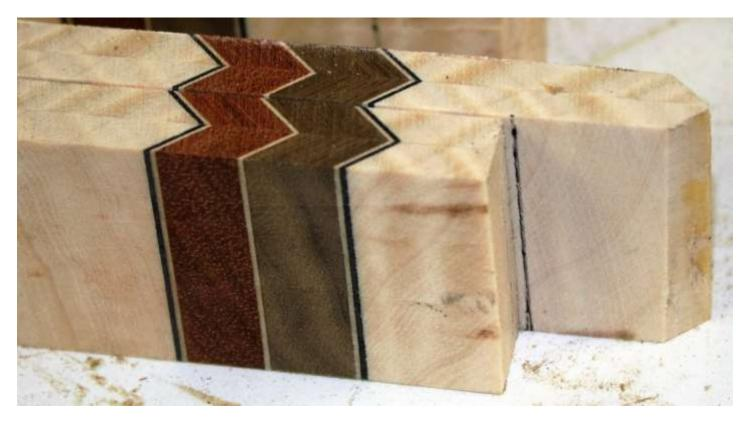
I cut these on the band saw. I think it's a bit safer to cut smaller pieces this way and then sand the edges to the desired length as shown below.
