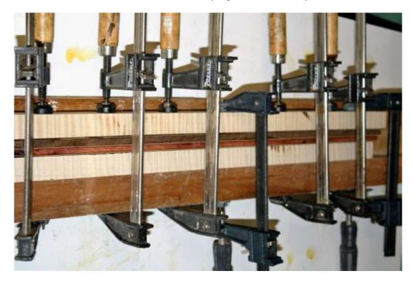
I like to use lots of screw clamps for nice tight even pressure. My clamping jig is just a couple of straight boards screwed together. I've also coated the jig with packaging tape to facilitate easy clean up of excess glue and if it gets to be too much trouble I can just peel the tape off and reapply.
