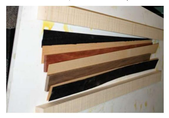
Below you can see my clamping jig and the boards being glued. I use an applicator roller bottle for an even coat of Titebond Original glue.
