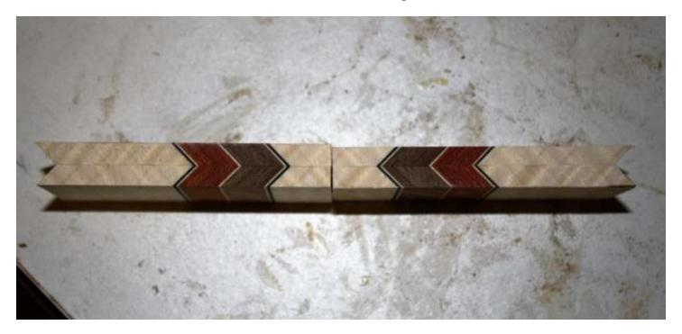
Below-sanding the section flat on both sides. Now this piece is ready for gluing the next layer.
