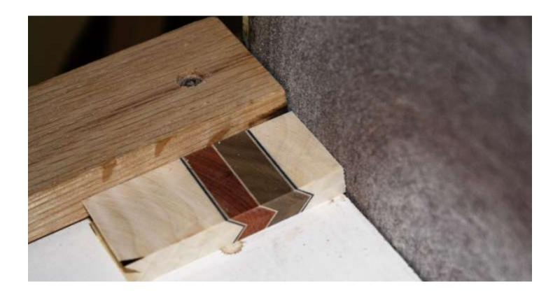
Now that I have two halves cut and sanded I can glue these together. They will be sanded flush after the glue dries so if they are of slightly different thicknesses it's not a big deal-just make sure the centers are aligned.
