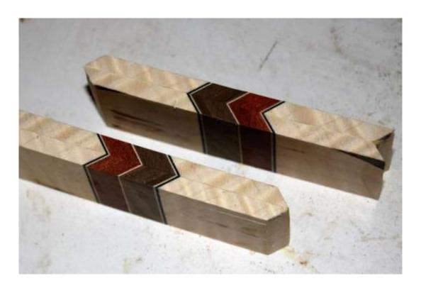
Above are the first two pieces of the design ready to be cut to create the middle section. And below I have cut the end off one piece and marked another. This is where you have the option of lengthening or shortening your pattern. Just cut off what you need for your design.
