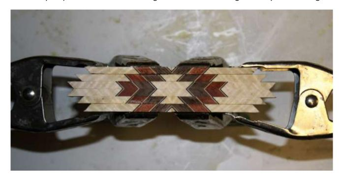
The photo below shows the final two maple pieces glued in place, completing the design. When the glue has dried I'll sand it smooth all around and cut it for inclusion in my feature ring.
