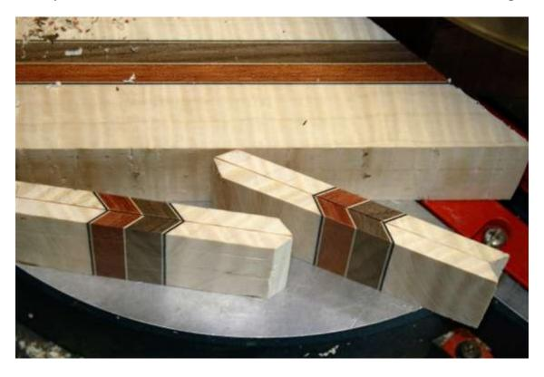
My next step is sanding one side of each piece. I don't sand both sides because after gluing the two pieces together I'll sand them both flush at the same time.
