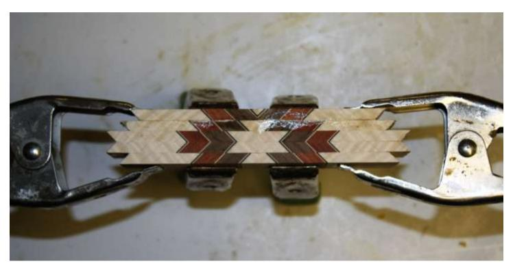
Below is the final design layer added. Now after I sand the layers flat I'll cut a couple of pieces of curly maple to sandwich the design and then cut to length for my feature ring.
