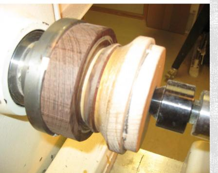
Prepare a waste block and glue on the bowl blank bottom.
