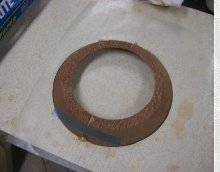
Gluing the rings using a rub joint reinforced with duct tape.
