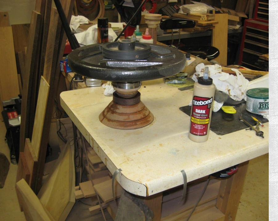
Continue the process until all the rings are stacked into the final blank.
