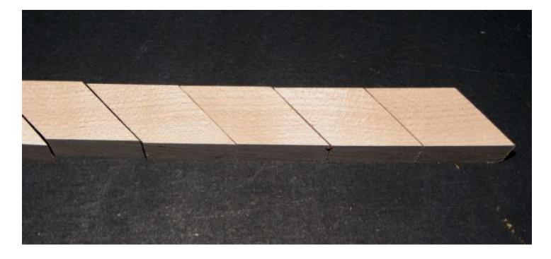
These maple pieces, also cut at 45 degree angles, will be sanded and glued to each side of a segment as shown below. I cut them slightly over length and sand back down to flush. These are just assembled with a rubbed glue joint to squeeze out excess glue and no clamping. If you need to clamp, by all means find a way to do it.
