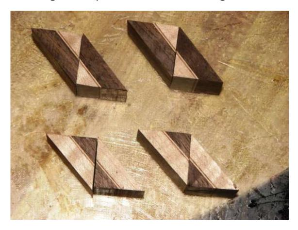
My next step is cutting strips to fill in the edges so I can have enough wood on the sides to cut my pieces into segments.
