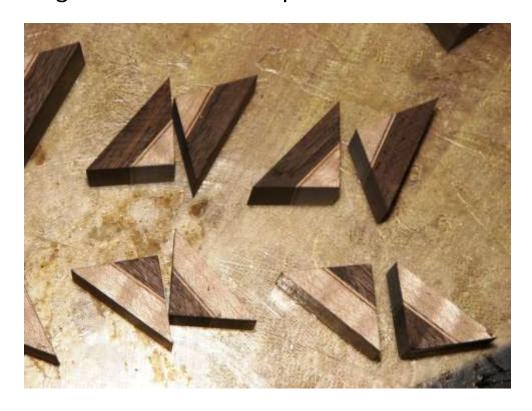
By lining up the edges of the woods or the veneers, I can sand and glue the pieces to form the hourglass.
