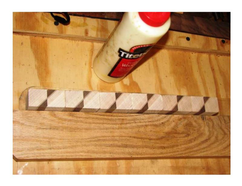
At this stage I cut a segment from a waste piece of wood the same dimension as the final segment size. I use this as a template to mark my new 'segment board' so I can cut the segments on my table saw sled the same way I cut pieces for any other ring.
