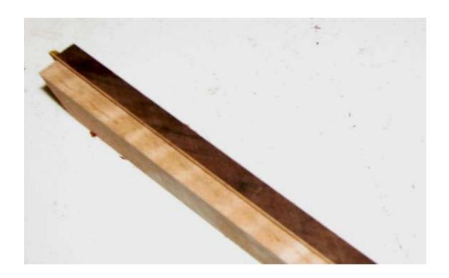
Then I cut 45 degree wedges from the laminate on the miter saw.
