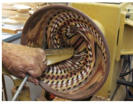
Start turning the inside one or two layers at a time checking wall thickness as we go Continue turning and checking wall thickness
