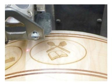
The laser acts just like a computer printer with laser unique parameters set in printer setup. For engraving the laser power and speed are specified which vary according to wood and desired engraving dept. For each segment, the laser pointer was set to the upper left segment corner and the appropriate PDF file was sent to the laser and segment was engraved.
