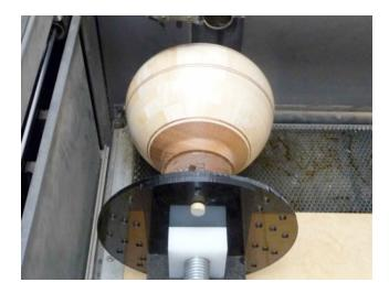
The laser is aligned to the bowl via a pointer that was placed in the upper lefthand corner of each segment.
