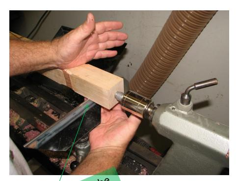
Toolrest is up under the blank, holding it square height and maintaining height
