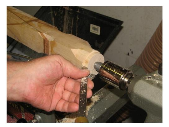
Reverse the blank in the lathe, and omitting the creation of the tenon, repeat the centering process on the other end of the blank.
