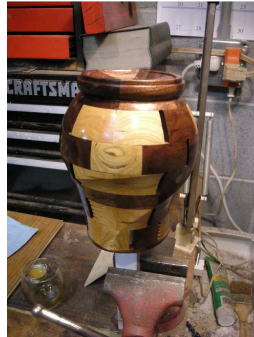
This was after multiple coats of finish were applied. The inverted drying was done for the outer surface
