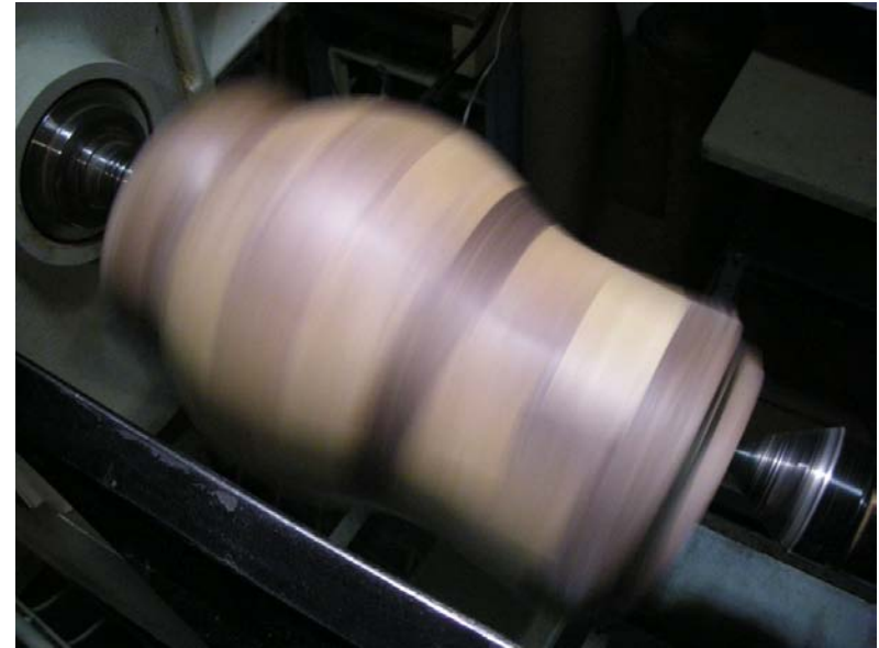
The part 'wobbles' during off-axis turning
