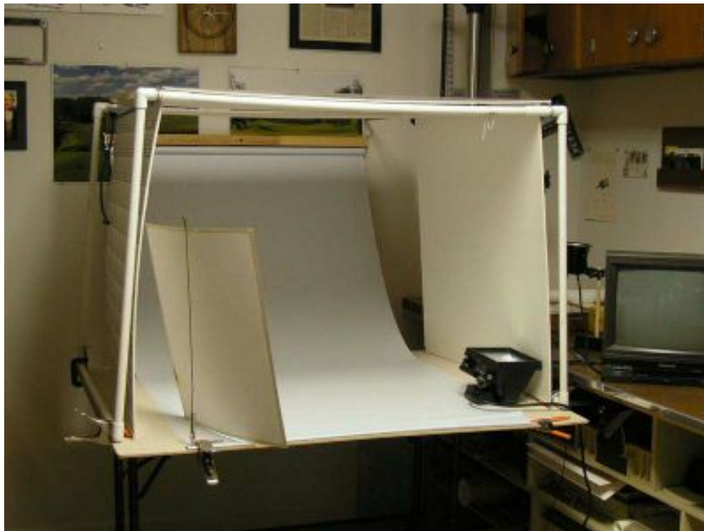
Photo 1 - Frame is ½" PVC pipe, the sides measure 34"x34" and top is 44" wide. Backdrop is white vinyl roll-up window shade. I often plug camera video into this monitor for enhanced view of camera image.
