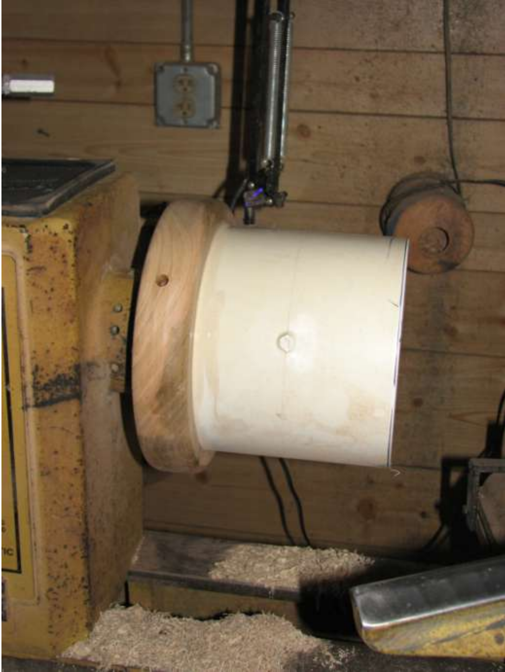
The chuck mounted to the lathe ready to be trued.
