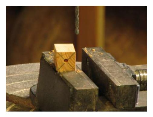
Close up of accent piece. Use a very sharp bit for this. The bit has a tendency to drift with the grain.
