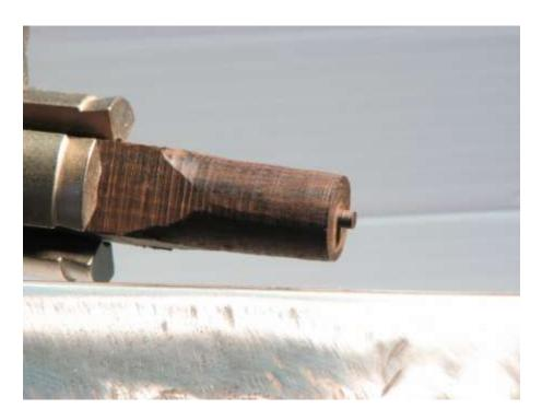
Here I've turned an 1/8" tenon on the end of my pen blank. Make sure you have a very flat surface around the tenon to mate up to the middle section. I also leave tiny grooves in the tenon to help give the glue something to grab.
