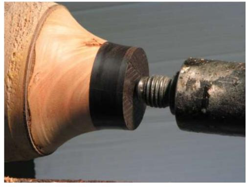
Turn the base round and just slightly larger than your finished diameter. Here, I've cut the waste block back in a nice sweeping arch-just because it felt so good to keep the cut going.
