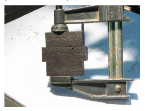
Glue the sections together. Notice the line I've drawn for reference. Try to keep the grain orientation the same for a more even look when glued together and turned. I usually use Titebond glue for this step.
