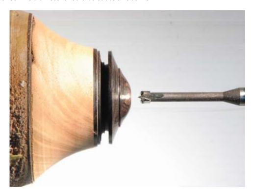
With the base completed, we can move back to the finial. Here we turn the middle accent piece and drill another 1/8" hole to accept the upper piece. I usually finish this section and then move on to the lower section.
