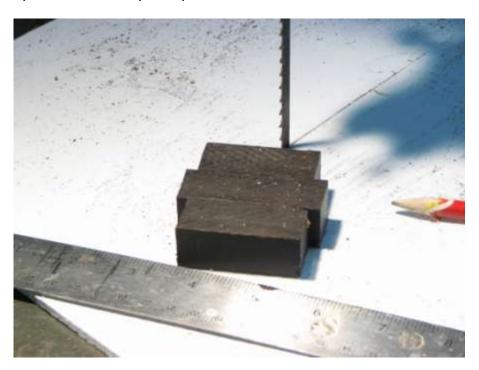
Step two is to cut the pen blank into 3 pieces to form the base. I will typically cut the center section just a bit longer thinking that I can get another millimeter of diameter if I need it.
