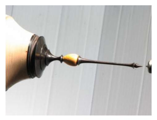
To finish the base, I put the whole thing in a long narrow vacuum chuck. A vacuum chuck of this diameter doesn't have much holding force, but it's enough for some light cuts and sanding. I usually turn a couple of rings on the underside to show it was turned and maybe to sign it.
