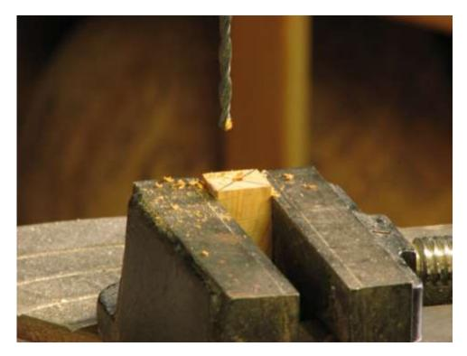
Drill an 1/8" hole in the accent piece of wood. Not all the way thru –just enough to accept the tenon. Again the surface should be flat to mate up to the bottom finial section perfectly.
