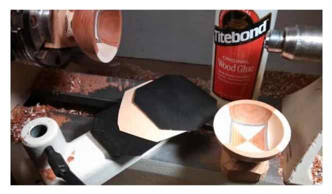
Be sure to apply good pressure on the veneers and keep them clamped till the glue is good and dry.
