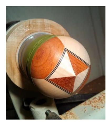
Here's a better shot of the PVC chuck. I cut a round groove in the wood block to accommodate the coupling and attach it in with Polyseamsealan adhesive caulk that I use for lots of stuff. Very good adhesion. I think the clear has better holding power but have no scientific proof. It's not a bad idea to sink the coupling deep enough to also get a few screws thru the wood and into bottom of the coupling for extra strength.
