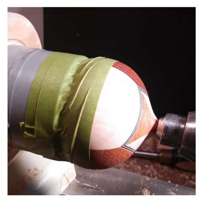
Here you can clearly see the PVC chuck and tape job. Once the ornament has been taped tightly, the tailstock can be pulled away to provide ample room to finish the bottom.
