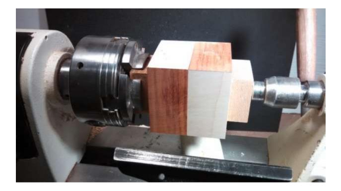
Step 8- Now we can start turning the segments into the shape we want.I turn only the middle to final shape and leave the ends kinda thicker to give me more stability when I hollow the insides.
