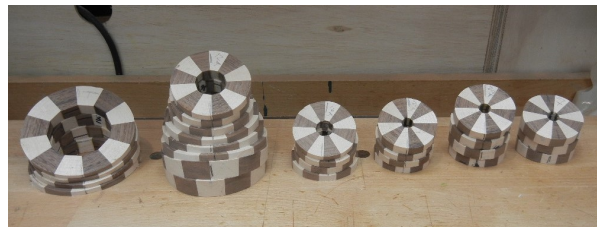
Ready for glue up. Notice I rounded the rings by eye on the disk sander to reduce the amount of shaping after glue up
