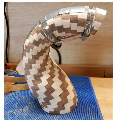
Ready for final shaping Mostly with hand held right angle sander
