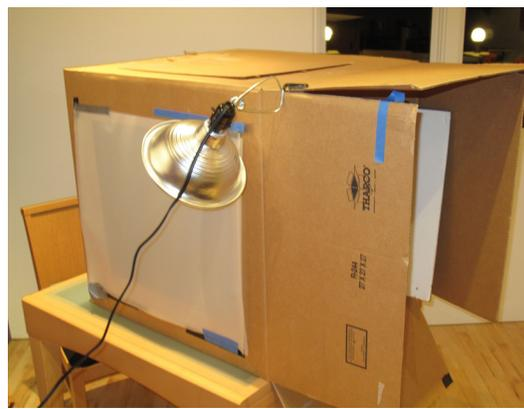
I keep this box on a shelf in my shop. It doesn't allow for much adjustment but it is a super fast way to get a quick shot. The box is 27" x 27" I placed a graduated back-drop inside and cut a hole in the left side with diffusion taped over it. It doesn't take a fancy light to make this work. I will talk about the white reflection card later.
